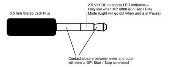
The GPI Function can be set to either control Play & Pause or Record & Pause. To select the GPI Function you require, start with the LCD Display showing the General Display
